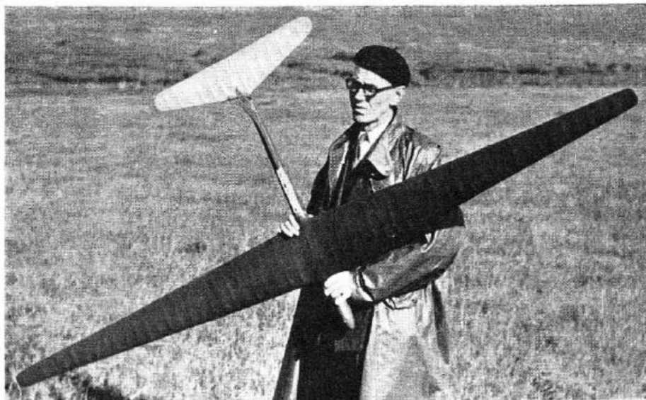
Age Høst-Aris—oldest Danish aeromodeller at ripe old age of 59 !—has been in Danish National team since 1946. He is seen here with his latest A2 Høst 29. DT fuse is placed in a metal channel located on fuselage just behind the wing.
