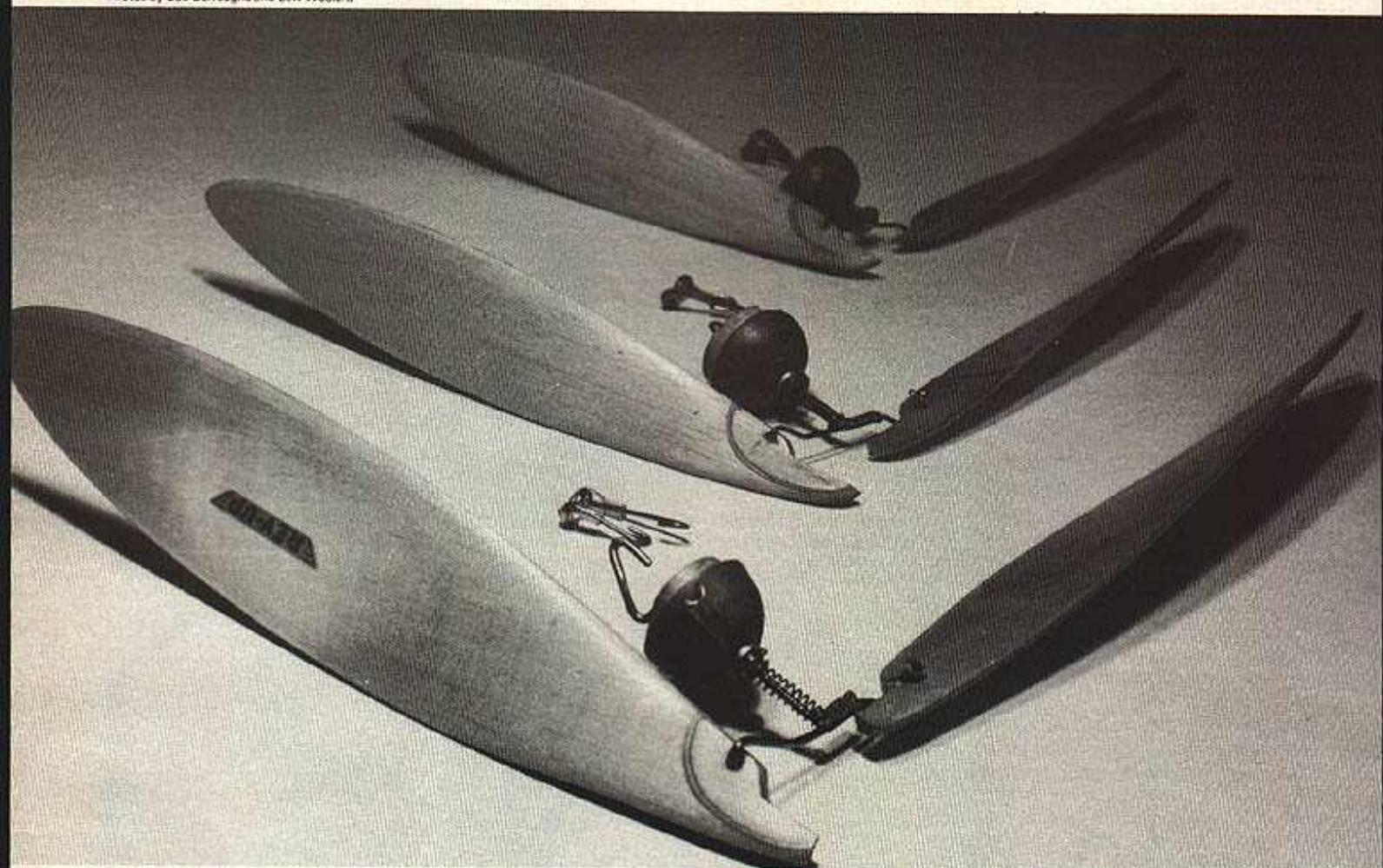
Less work, and cheaper, than carving rubber-model props, these sturdy blades will spare you the soul-shattering experience of 'self-destructing' props when striking the ground. ■ Jim O'Reilly
