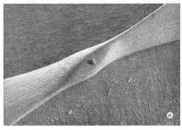
Fig. 17: The slightly hollow surface of the rear faces of the blades is now smoothed out with the help of a piece of sandpaper wrapped round the finger. The leading and trailing edges are sanded to a smooth curve outline, the former with a rounded cross section, the latter tapering away to 1/16 in. thickness.
